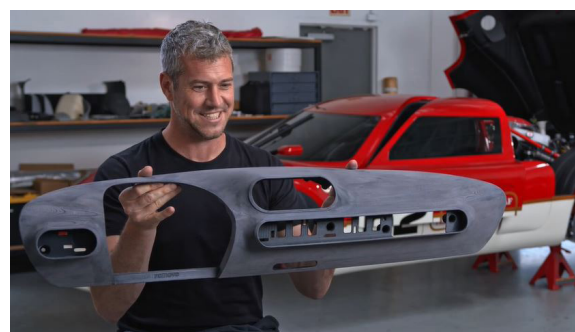
The 3D printed dashboard instrument panel will be covered with leather before installation.
